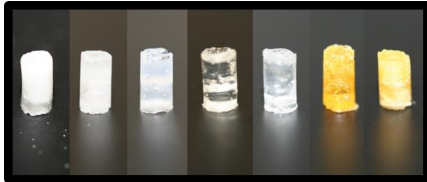
Figure 5.2. Cylindrical mechanical testing samples of PSIM copolymers and blends. From left to right : mPEG (5kDa), mPEG (2kDa), PLA(5k), PLA(2k), PLA(550), PSIM(5k), 80:20 PSIM(5k):PLA(5k), and 60:40 PSIM:PLA.
